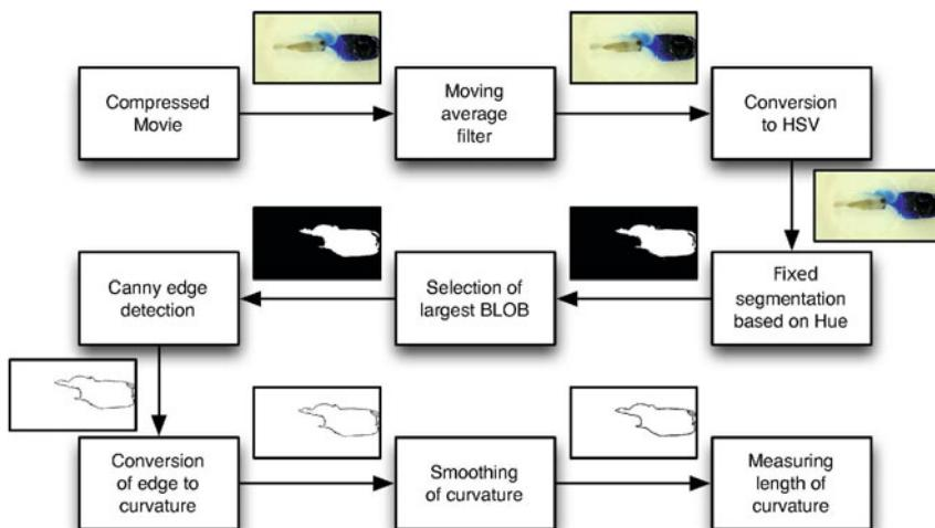
**Fig. 3.** Processing chain for dye mixing videos of the mixing array
