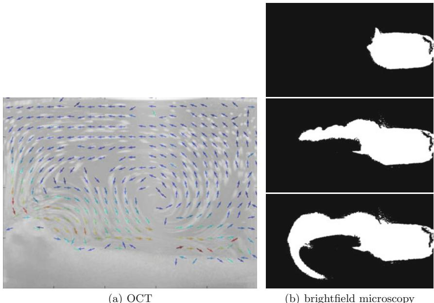
**Fig. 2.** Image processing. The velocity vector field is superimposed on Fig. 1(a) [5]. The vectors indicate direction and color indicates velocity. Velocity is scaled from blue ( $> 0$  mm/s) to red (300 mm/s). In video microscopy, dye is segmented by static thresholding in HSV colorspace.
