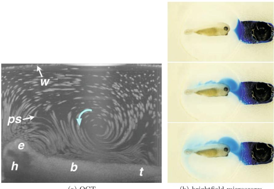
**Fig. 1.** Multi-modal source data. The projection over time of OCT images shows a water/air barrier (w), streak lines produced by the particles (ps), and the animal (eye (e), head (h), body (b) and tail (t)). The blue arrow indicates the direction of flow. In video microscopy, the blue dye is clearly visible.
