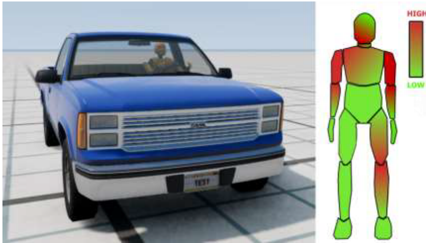
Figure 2. Left: Real-time render of BeamNG.drive with dummy placed on driver seat Right: Visualization of a possible representation of forces enacted on dummy during crash.
