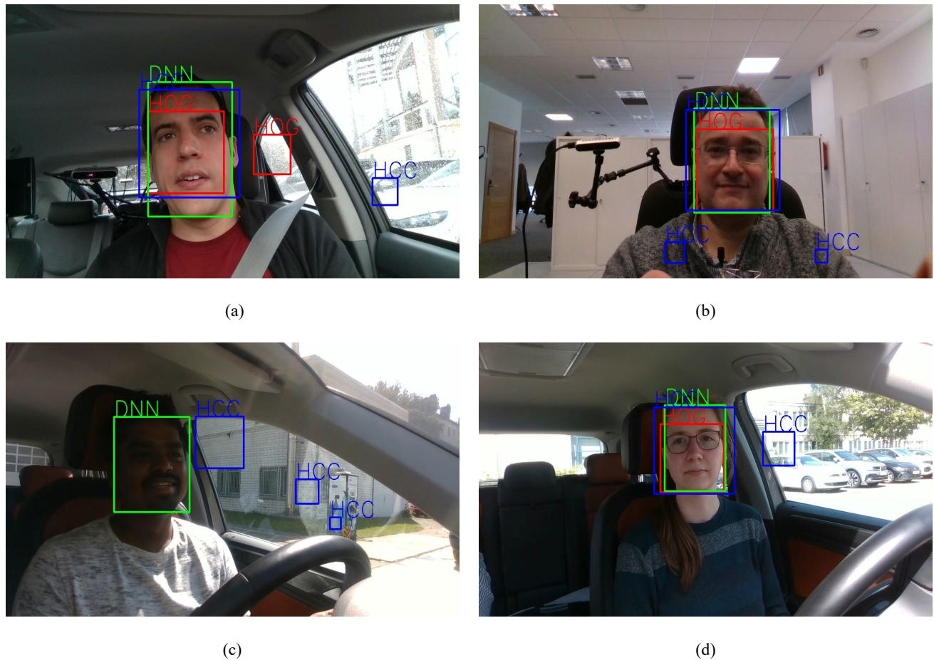
Figure 2. Example frames before post-processing a-b) stem from DMD, and c-d) stem from our own self recorded dataset. Red, blue, and green color boxes indicate HoG, HCC, and DNN respectively.
