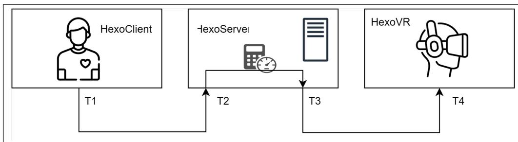
Figure 5: Time points  $T1$  to  $T4$  correspond to the individual modules.  $T2 - T1$  represents the transmission duration from HexoClient to HexoServer. The calculation duration of the QRS detection in HexoServer is  $T3 - T2$ . Finally, the transmission duration from HexoServer to HexoVR is  $T4 - T3$ .
