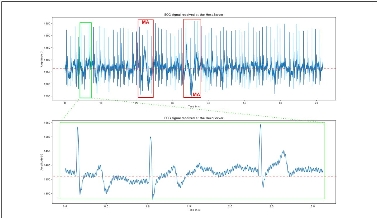
Figure 3: Received ECG signal from HexoClient. The upper graph displays the 70s signal, while the lower graph shows a 3.5s segment of the signal (marked with the green box). All components of the EKG are discernible in the signal, but there are also some artifacts present. It contains a baseline shift of around 1370 mV (red dotted line), motion artifacts (red boxes, marked with MA), and the typical 50 Hz noise.
