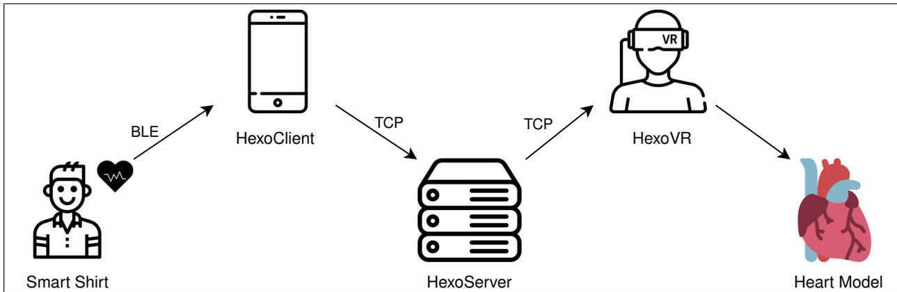
Figure 1: The HexoMonitoring application consists of three components:(i) HexoClient: This component records the ECG via Bluetooth Low Energy (BLE) from the Smart shirt.(ii) HexoServer: Running on a Desktop PC, this component detects the heartbeats.(iii) HexoVR: Also running on the same PC as HexoServer, this component visualizes the data in the VR environment.
