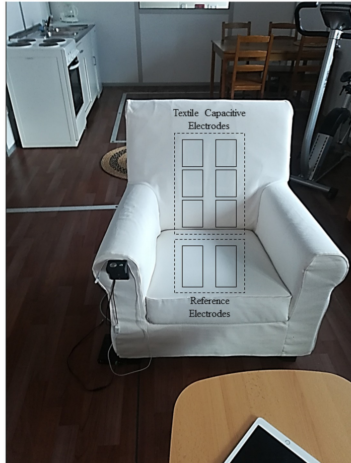
Fig 1. cECG armchair with capacitive electrodes.
