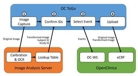
Figure 2: System architecture and workflow of OC ToGo with ID detection.
