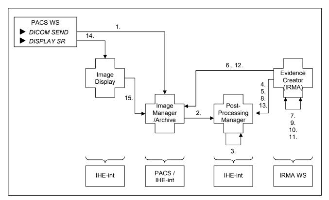
**Figure 2:** IHE intermediate stage workflow for support of hanging by IRMA. Shown are direction and order of actions/communication (arrows) between the IHE actors (crosses) on the different machines (rectangles).
