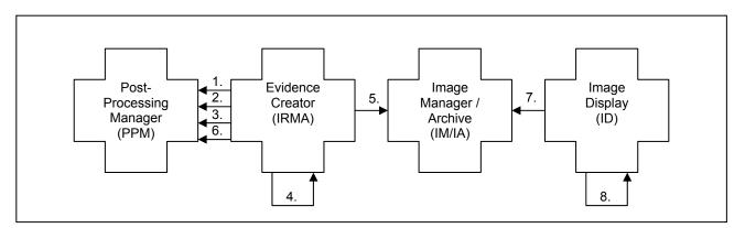
**Figure 1:** IHE compliant workflow for support of hanging by IRMA. Shown are direction and order of actions/communication (arrows) between the IHE actors (crosses).
