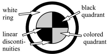
**Figure 1.** Design of optical landmarks.
