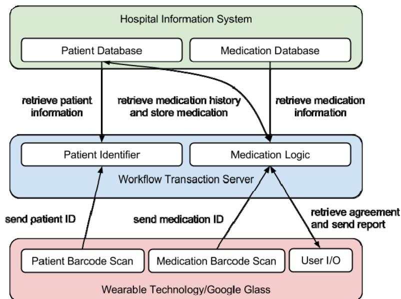
Figure 3. Workflow integration of wearable technology and transaction server into the current hospital information system. The arrows represent the data flow.
