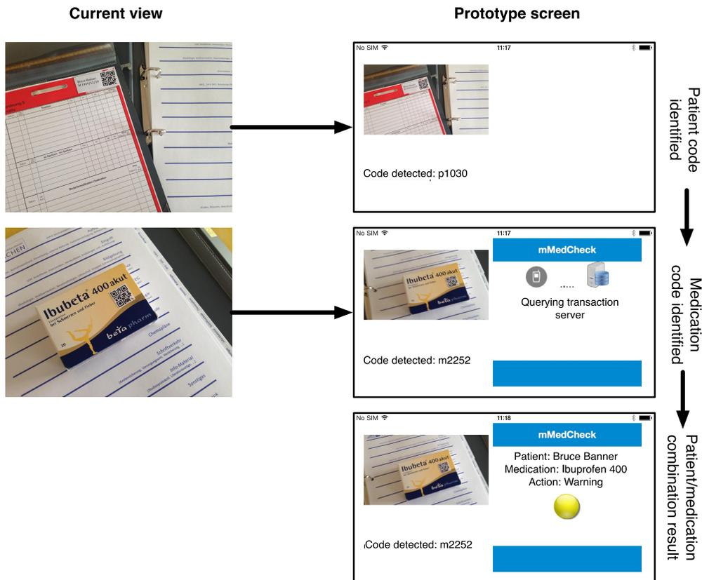
Figure 2. Sample workflow of medication performed with current prototype. On detection of both a patient and medication code, a query is submitted to the transaction server and a color-coded result is returned.
