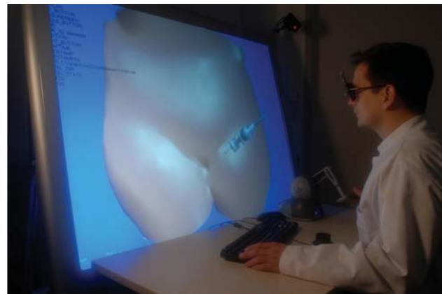
**Fig 6** VR-based setup of the RA simulator application. The trainee controls the virtual needle through a PHANTOM Omni Haptic device.
