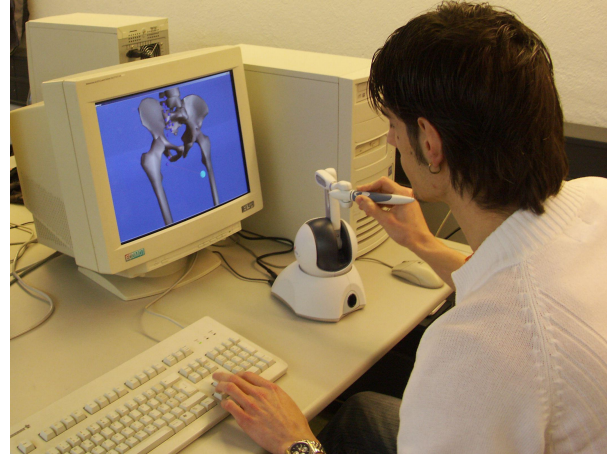
Figure 3. The modeling system allows for the interactive editing of control points. DICOM datasets can be co-located to verify the local anatomical setup.
