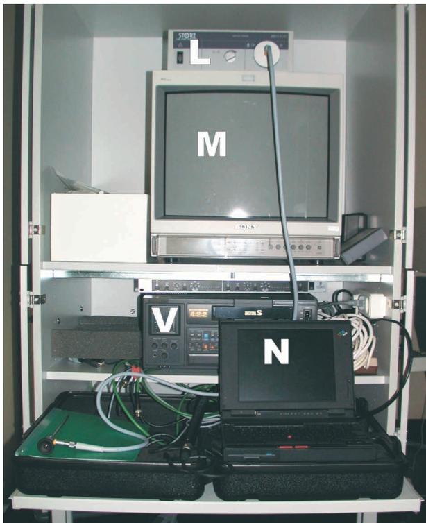
Fig. 1. The videolaryngoscopy set-up, consisting of a xenon light source (L), video monitor (M), digital video cassette recorder (V), notebook computer for storing white balance values (N) and CCD video camera (not pictured).
