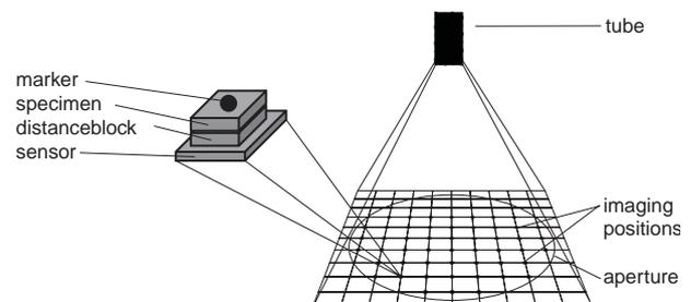
Figure 2 Experimental setup for raw data acquisition
