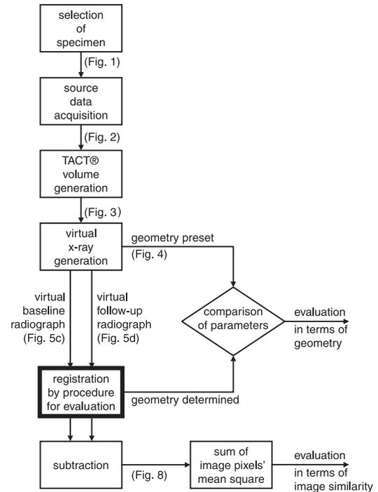
**Figure 7** Flowchart for the performance evaluation of registration procedures by means of virtual radiographs computed from high-resolution TACT volume data
