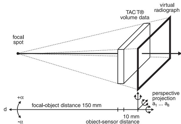
Figure 4 Geometry for simulation of X-ray projection. The symbols  $d$  and  $\alpha$  refer to Table 1 while the parameters  $a_1$  to  $a_8$  are defined in Equation (1)
