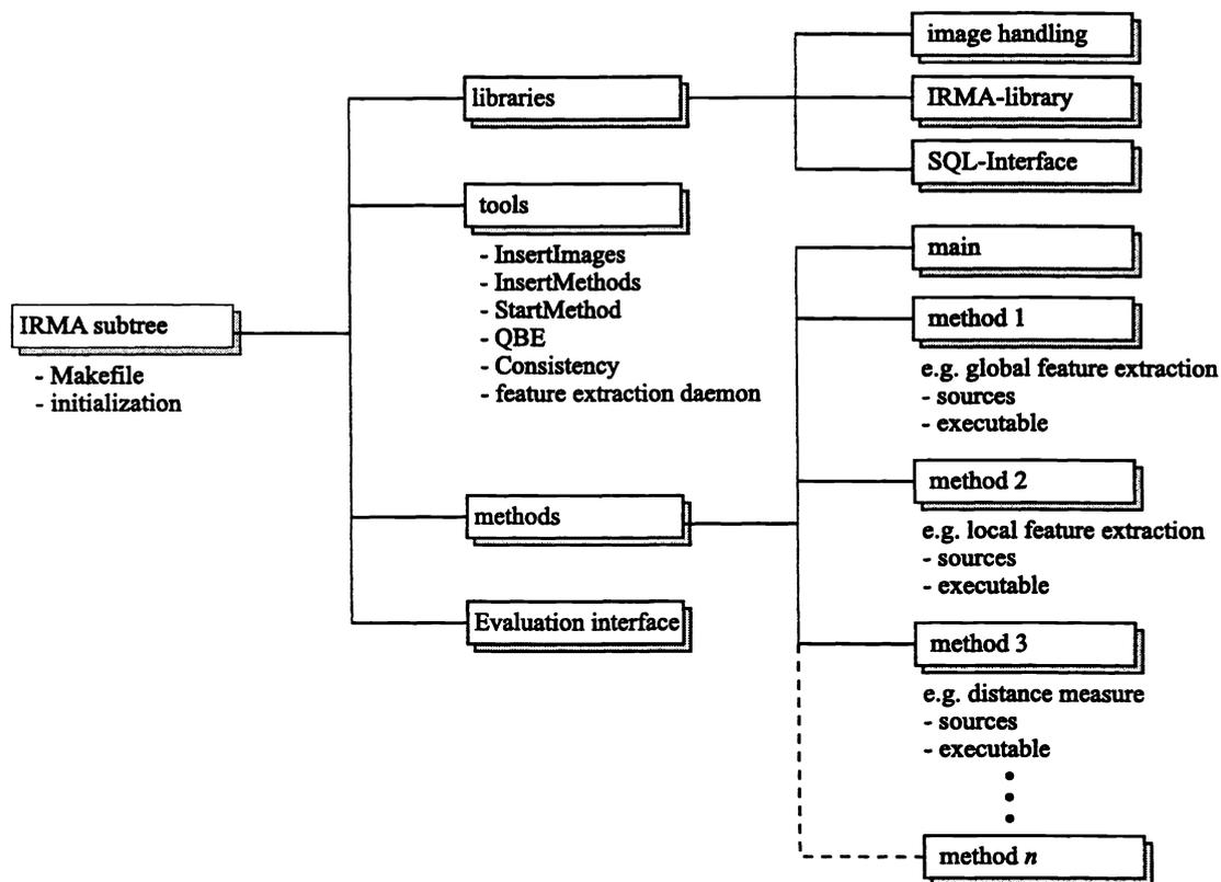
Figure 2. The installation subtree of a development site.
